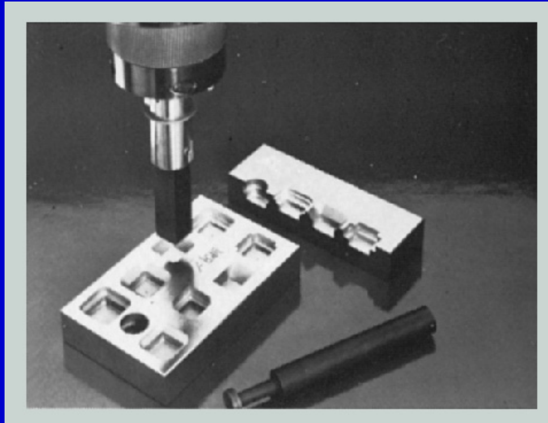
FIGURE 9.34 Stepped cavities produced with a square electrode by EDM. The workpiece moves in the two principal horizontal directions, and its motion is synchronized with the downward movement of the electrode to produce various cavities. Also shown is a round electrode capable of producing round or elliptical cavities. Source: Courtesy of AGIE USA Ltd.
