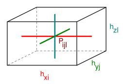
• Each node is considered as "homogeneous" in terms of material and the neutron flux is approximated in it by a second order polynomial in the different directions
